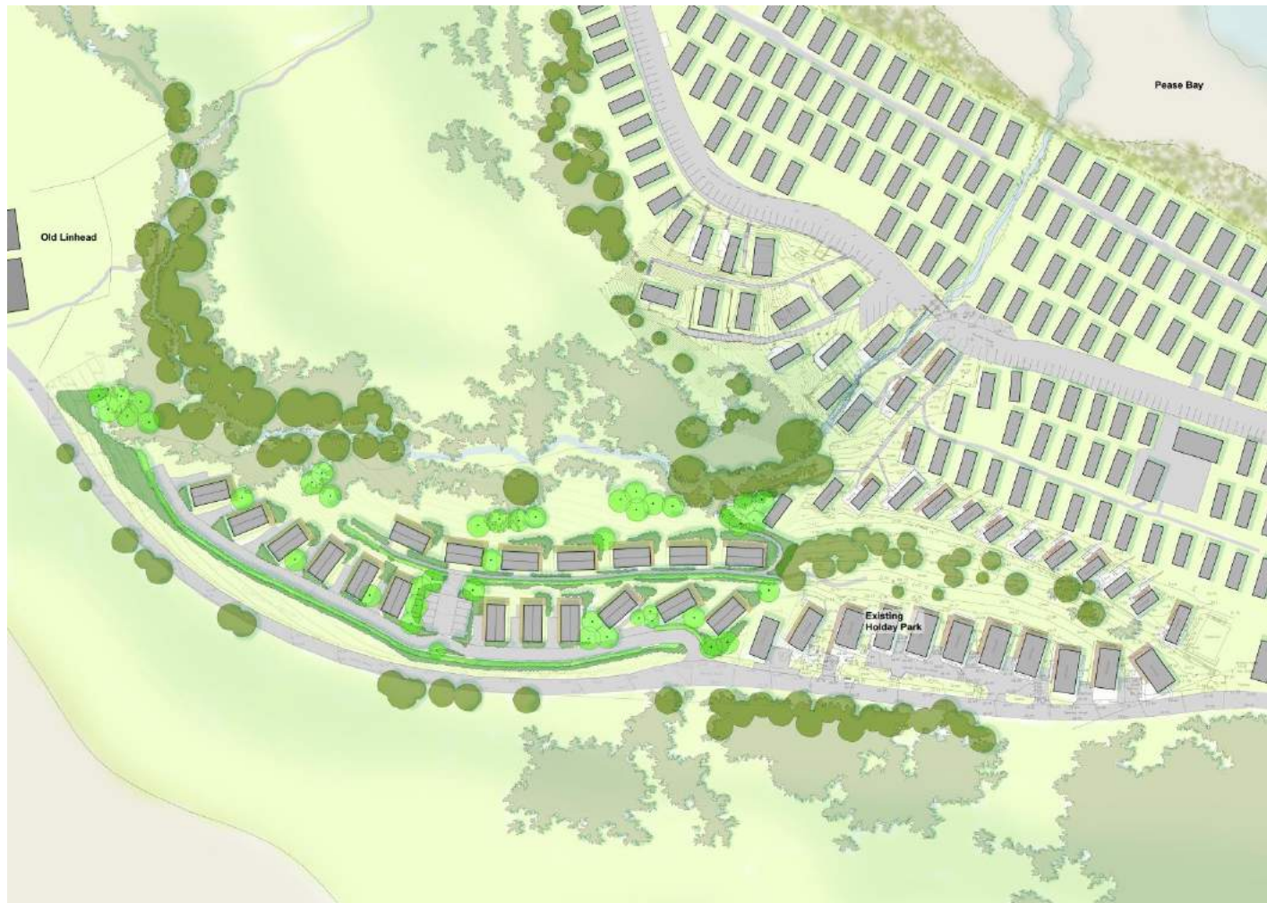
Figure 5.2 Proposed mitigation includes extensive tree and shrub planting, the use of a green retaining wall system, and adjustments to the layout to provide additional space for roadside planting. A fully annotated version is provided in drawing 02, Landscape Plan.
